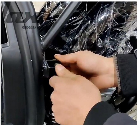
7: Install the rear wheel shock absorber and tighten the screws
