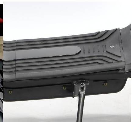
10:After installing the pedal lock, secure the pedal. The battery compartment below the pedal can be purchased with additional batteries to increase mileage.
