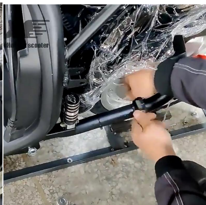
7: Install the rear wheel shock absorber and tighten the screws
