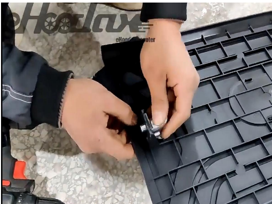
10:After installing the pedal lock, secure the pedal. The battery compartment below the pedal can be purchased with additional batteries to increase mileage.
