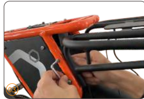
Use an M6 Allen wrench and a 10mm wrench to tighten and secure the rear rack
