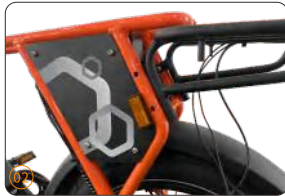
Align the rear rack with the screw holes and attach the screws
