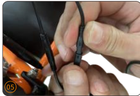
Connect the rear light power line (strictly follow the directional arrow on the line)
