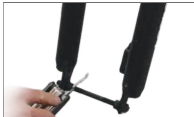
01 Release the front fork guard bar
