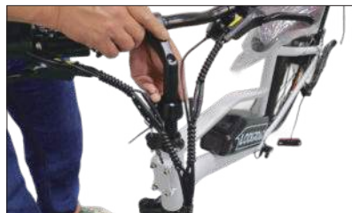
01 Insert the handlebar into the handlebar holder.
