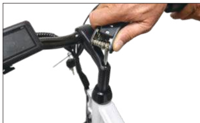
02 Lock the handlebar fixing screws to secure the handlebar.
