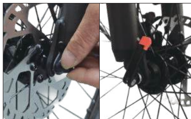
05 Install the front wheel onto the front fork, attach the protective screws, and lock the front wheel axle.
