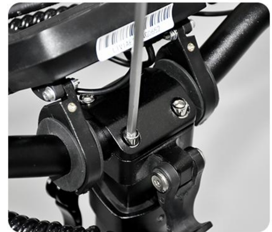
5. Reattach and tighten the screws
