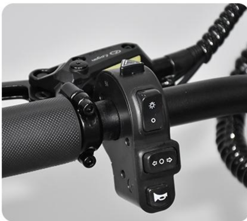
6. Check whether the brake handle, headlight switch, dual drive switch, and instrument are fixed
