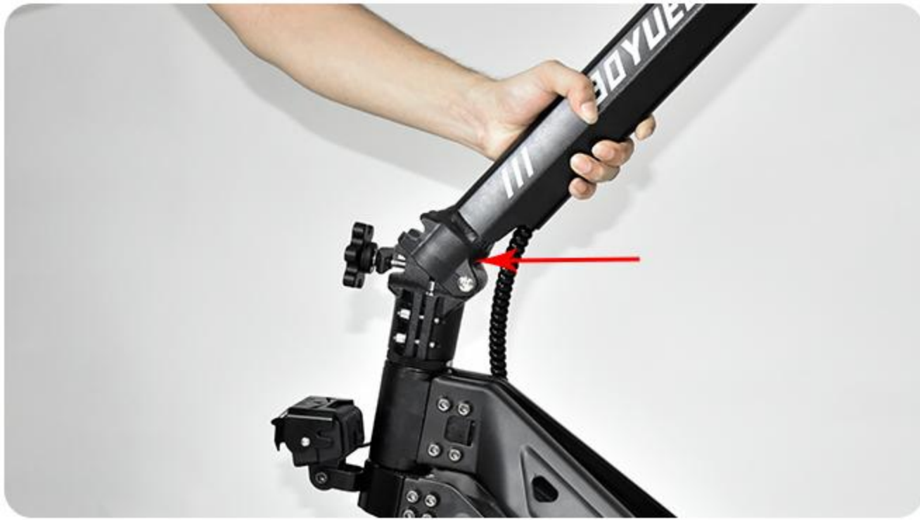
1. Raise the handlebar until it locks into place
