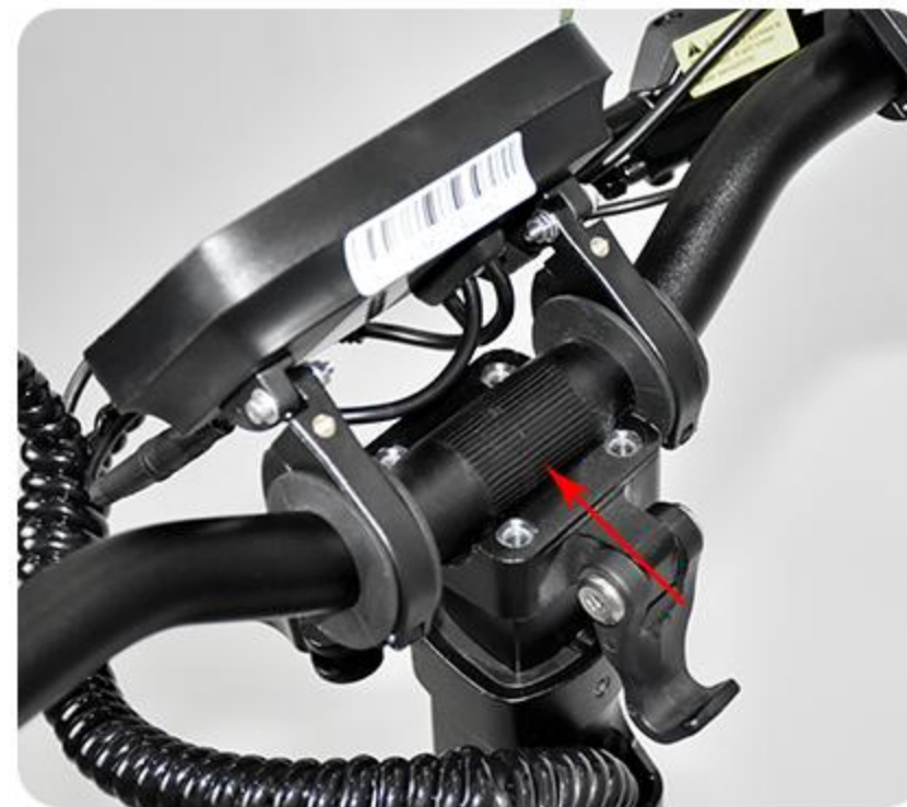
4. Insert the handlebars into the corresponding slots
