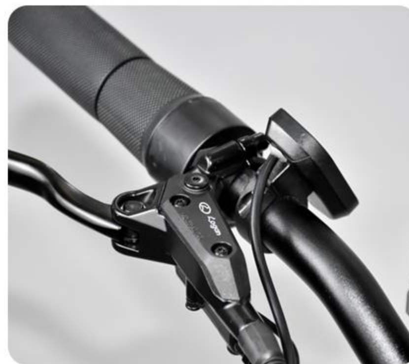
6. Check whether the brake handle, headlight switch, dual drive switch, and instrument are fixed
