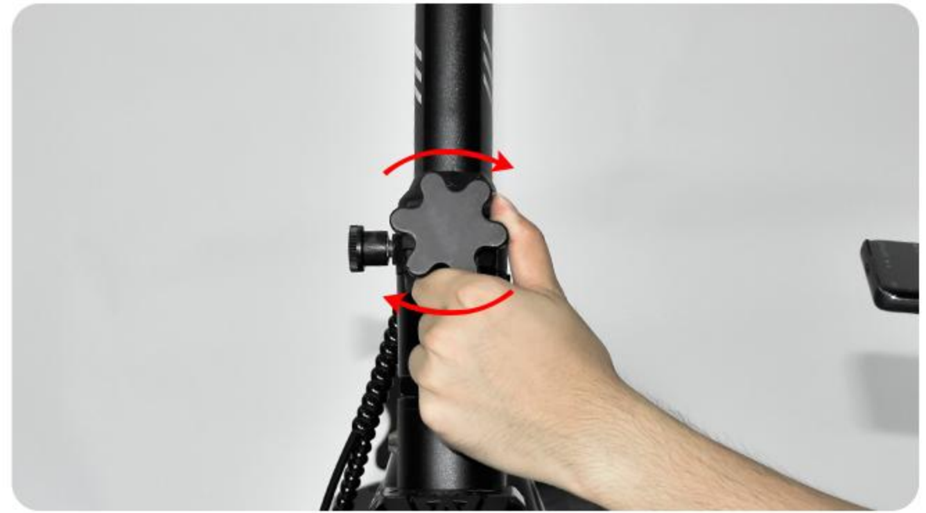
2. Turn clockwise to tighten and lock the handle
