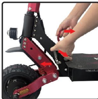
2. Press the silver snap in the direction of the arrow so that the silver snap completely leaves the lower slot and pull the red folding stick in the direction of the arrow.
