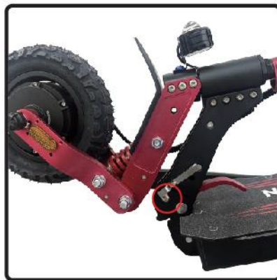
4. When the silver snap is catching the upper slot, the folding is completed.
