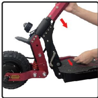
3. Lower the pole in the direction of the arrow.
